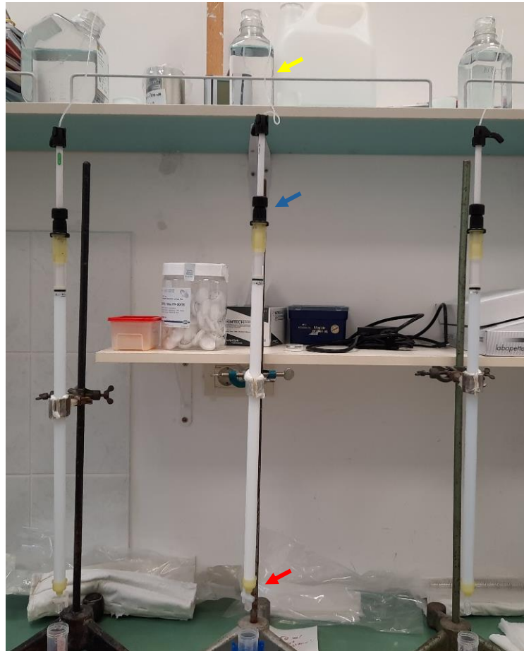
Figure 9. Display of in-house size-exclusion chromatography (SEC) set-up for exosome isolation. SEC was performed on glass chromatography columns equipped with porous polymer bed support at the bottom of the columns (red arrow) and packed with Sepharose CL-6B, Superose 6PG. and Sephacryl S-400. Elution was driven by gravity flow, and the eluent was delivered continuously from the mobile phase reservoir (yellow arrow) to the column through a tube connected by an adaptor (blue arrow).
